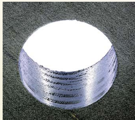
hole exit in unidirectional CFRP hole d = 6.35 mm
